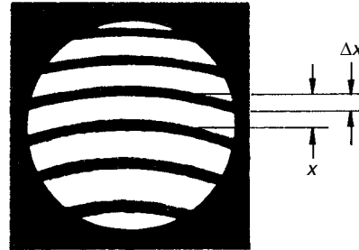
Fig. 1 Evaluation of the errors of a polished flat test surface by interference
