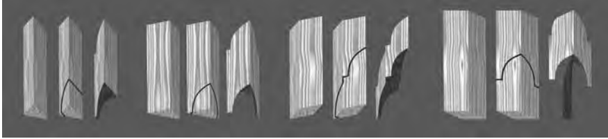
Fig. 3. The cuts of the four principle pieces, beginning with a triangular prism for the first two, and rhombic for the remaining two. The visible parts are shown in black
