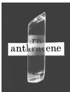
Fig. 1.4 An anthracene single crystal made by the Bridgman crystal-growth method, then cleaved and polished. The length of the crystal is about 2 cm and its thickness 1 cm. Along the direction of sight in this photograph, the c' direction, the strong double refraction is apparent. Image provided by N. Karl [1]. Cf. the coloured plates in the Appendix.
