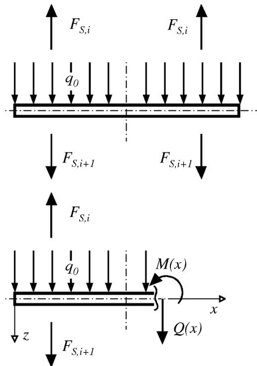
$$w'(x) = \frac{1}{EI} \left[ \frac{q_0 x^3}{6} - \frac{q_0 L}{2} \{x - a\}^2 - \frac{q_0 L}{2} \{x - (2L - a)\}^2 + C_1 \right]$$
