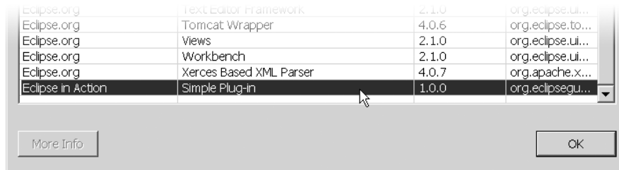
Figure 8.1 In the About page, you can click the Plug-in Details button to see the list of installed plug-ins. The Simple Plug-in shown here was discovered by the Eclipse Platform during startup.
