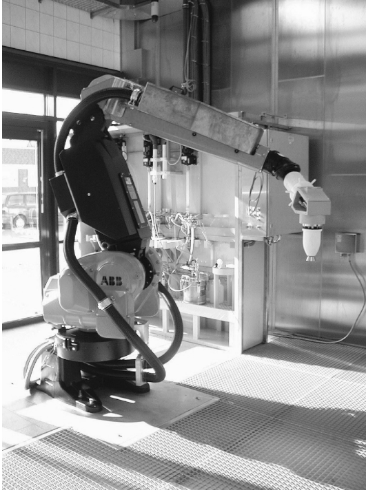
Fig. 1.5 Paint robot with electrostatic bell (source: BASF Coatings).
