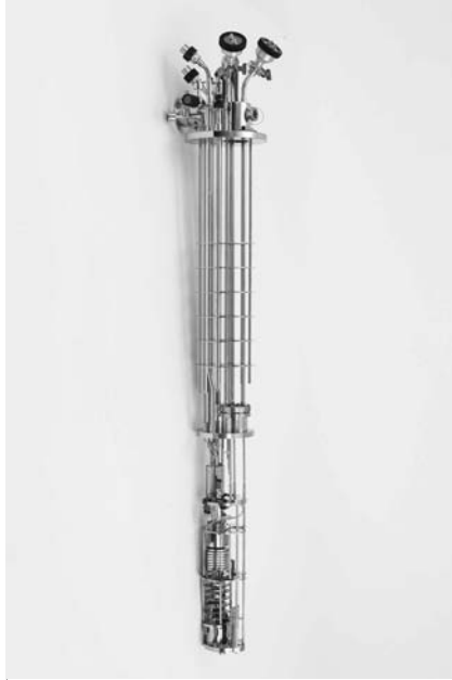
Figure 1.5: Mixing cryostat for cooling down to temperatures well below 1 Kelvin. The coldest end with the mixing chamber is located at the bottom. On the top one can see the flange for mounting into the cryogenic container, which can also be evacuated. (Photo: Oxford).
