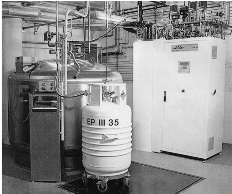
Figure 1.4: Modern plant for liquefying the noble gas helium. On the right one can see the liquefier; on the left, the storage tank; and in front of it, a transport vessel for liquid helium. (Photo: Linde).
