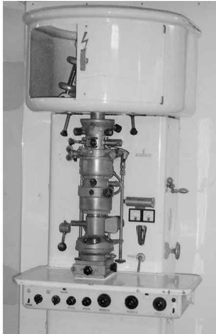
Figure 1.8: An early electron microscope from Siemens. (Photo: TU Berlin).
