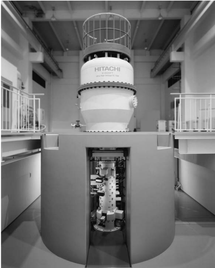
Figure 1.1: Modern electron microscope with an accelerating voltage of one million volts. (Photo: A. Tonomura).
