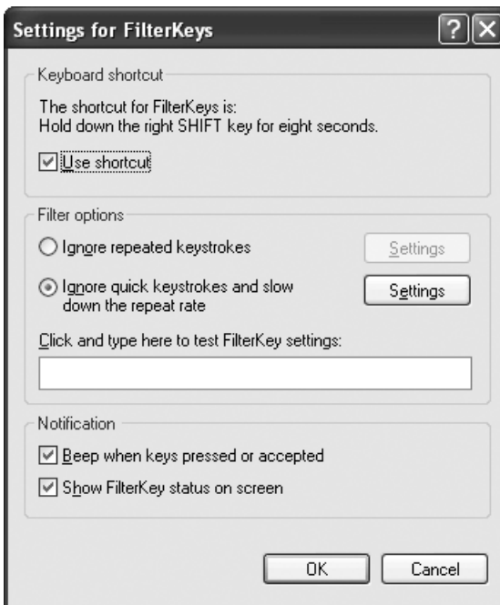
Figure 6-13. Define features such as the timespan between keystrokes using this dialog box.
