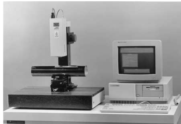
Figure 53. Assessment of surface texture on a diamond-turned component, within the range 5–10 nm R_q , utilising a non-contact optical instrument. (Courtesy of Taylor Hobson.)
