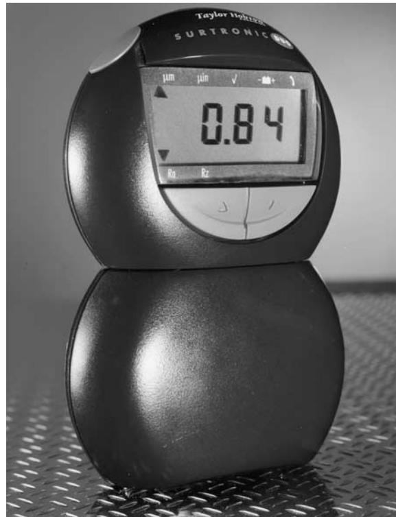
Figure 39. Portable hand-held surface finish instrument “Surtronic Duo” can be used at any angle/attitude. (Courtesy of Taylor Hobson.)
