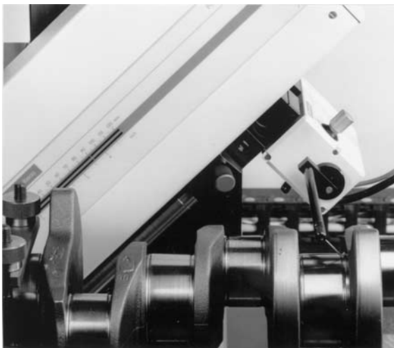
Figure 40. Form measurement with an inductive contour pick-up, including “customer-engineered” work-holding, for crankshafts. (Courtesy of Taylor Hobson.)
