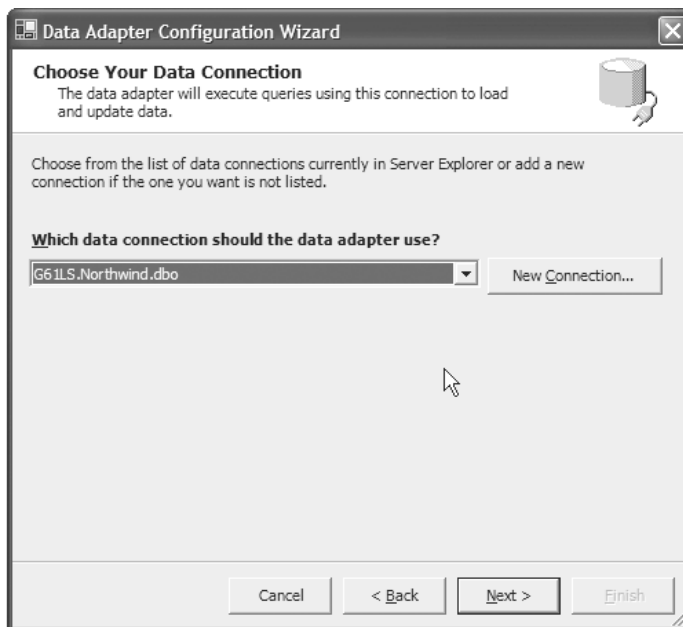
Figure 4-20. Choosing the Northwind SQL Server database in the Data Adapter Configuration Wizard
