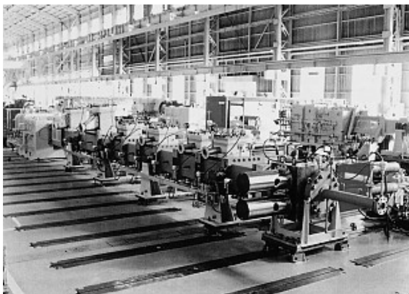
Figure 7.20 Intermeshing co-rotational twin screw extruder with 6 venting holes (JSW, TEX 250)
