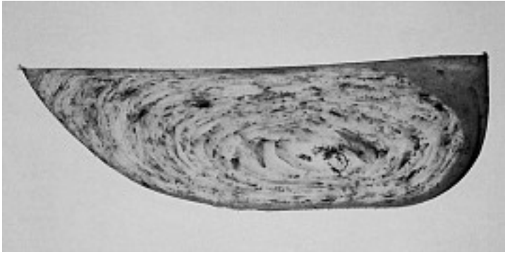
Figure 7.10 Solid phase deformation by strong shearing stresses in the melting region
