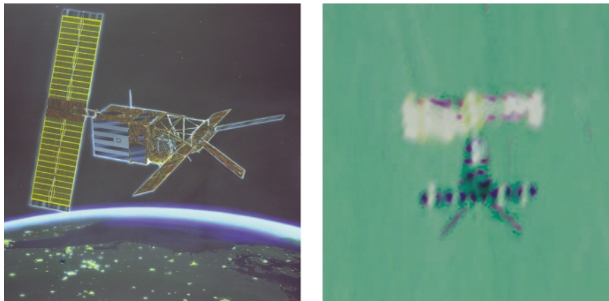
Fig. 1.3. The ERS-1 remote sensing satellite as seen by an artist ( left ; courtesy ESA) and imaged in orbit by the French Spot-4 satellite on May 6, 1998 over the Tenere Desert of Niger from 41 km altitude ( right ; photo credit CNES)
