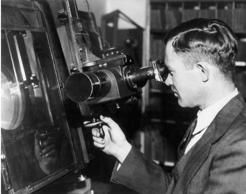
Fig. 1.6: Clyde Tombaugh in 1938 at the Zeiss blink comparator, which he used to examine pairs of photographic plates from the 13-inch telescope during his Pluto search. Following the discovery of Pluto, Tombaugh continued this dedicated but ultimately fruitless work in an attempt to find more distant planets. No discoveries were made. The large glass plates Tombaugh used each measured 14 by 17 inches (36 by 43 centimeters). (Lowell Observatory photograph)
