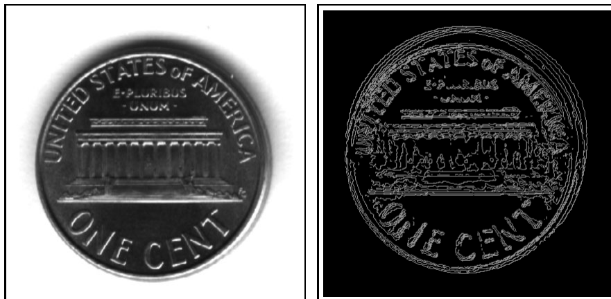
Fig. 2.13. Left: Original image, right: Boundaries estimated by rounding an MMS estimate from an edge model from Example 2.4.1
