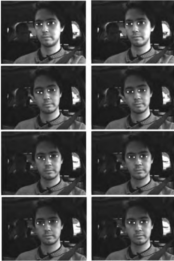
Fig. 3.12 Driver head tracking based on an existing method ( left ) and the proposed method ( right ). Video captured from UYANIK
