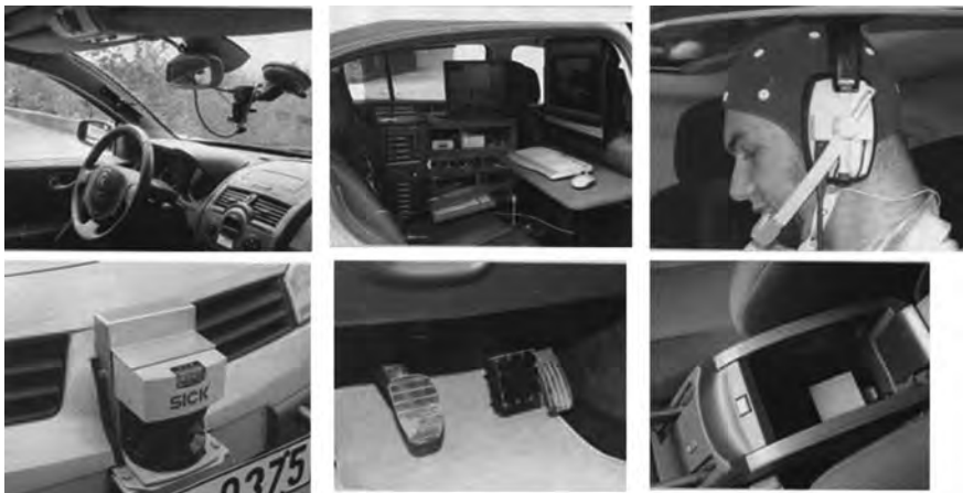
Fig. 3.3 Vehicle sensors: cameras, navigator area and instruments bench, laser range finder, 3D accelerometer, brake pressure sensor, microphone, and EEG cap (from top left clockwise.)
