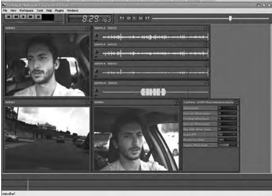
Fig. 3.5 Browser synopsis of the multi-channel multimedia display for Driver IF1014. Three video feeds and four audio waveforms together with steering wheel angle, vehicle speed, and engine RPM dials are included
